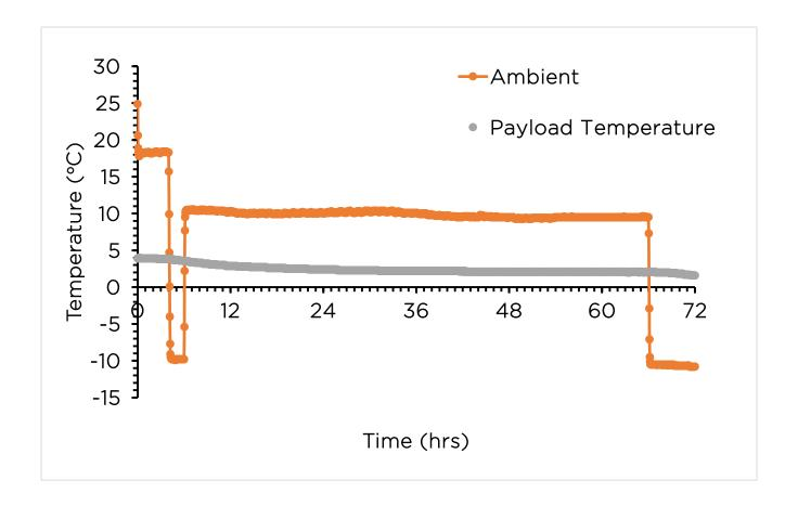
Average Payload Temperature: 2.6 °C | Test Result: Pass
