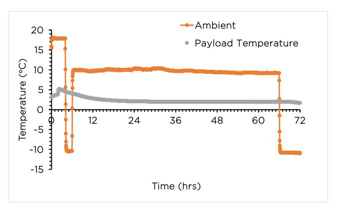
Average Payload Temperature: 2.55 °C | Test Result: Pass
