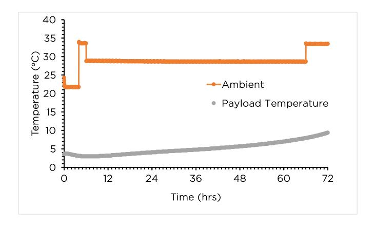
Average Payload Temperature: 4.1 °C | Test Result: Pass
