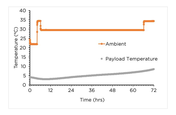
Average Payload Temperature: 4.3 °C | Test Result: Pass
