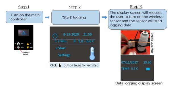
Sensor starting and cooler issue procedure.
