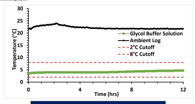
Minimum Payload Simulant Temperature: 3.6°C Maximum Payload Simulant Temperature: 6.5°C
