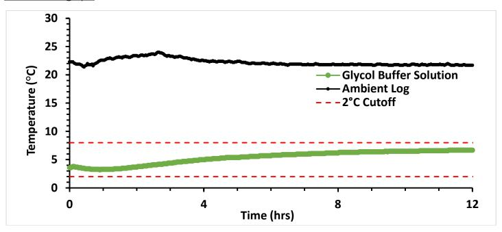
Minimum Payload Simulant Temperature: 3.2 °C Maximum Payload Simulant Temperature: 6.7 °C
