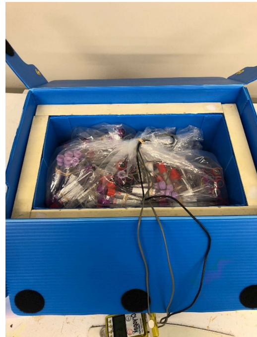
Figure 2. Bundled tube scenario used for 191-250 tube capacity. The photo above was taken prior to a thermal validation test and shows 250 tubes bundled in sets of five with data loggers attached.
