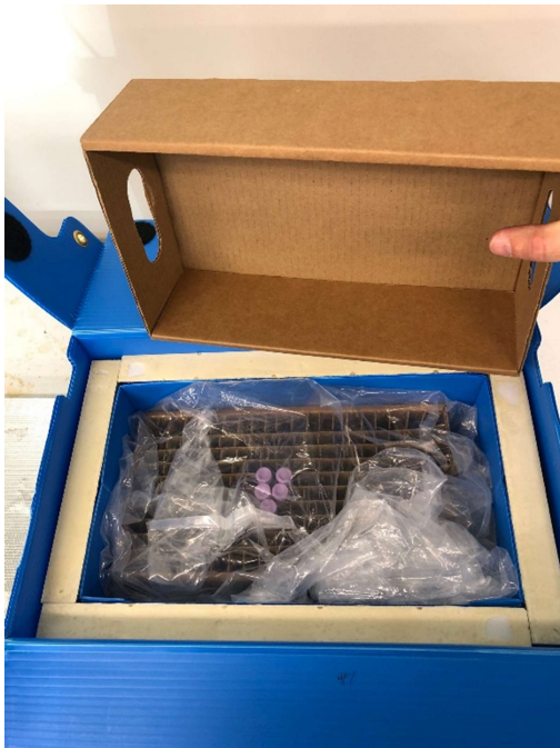
Figure 1. Tube rack scenario used for 1 to 190 tube capacity. The photo above was taken with the lid of the tube rack removed for clarity. The lid was placed on the tube rack for thermal validation testing.
