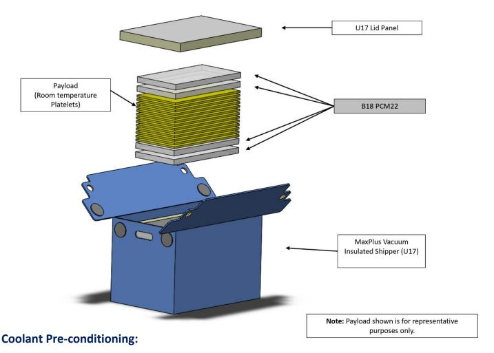
• Charge four B18 PCM22 coolant bottles in an incubator or controlled room temperature at (23°C  $\pm$  1°C) for a minimum of 24 hours.
